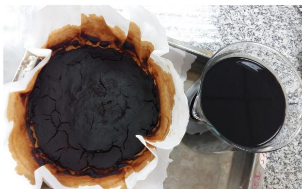
Figure 3. Removed impurities and liquor after the evaporation process.
